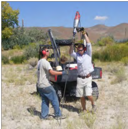
Figure 2. A 2-meter hollow rod is being inserted into the ground using a demolition hammer powered by an electric generator in the back of the ATV.
