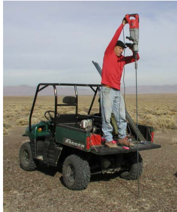
Figure 2. Hollow steel temperature probe being driven into ground with electric demolition hammer.
