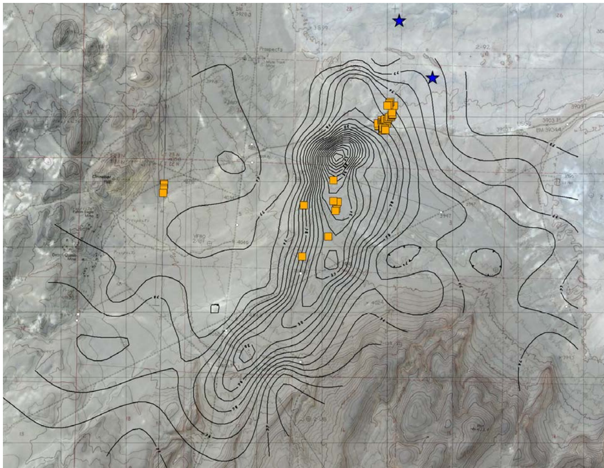
Figure 9. Location of carbonate tufa columns and artesian wells with respect to shallow temperature anomalies in the Desert Queen area. Yellow-brown squares are carbonate tufa columns. Blue stars are artesian water wells. Black lines are 1°C temperature contours. Black squares are 1km on a side. North is up. Background image is shaded topography superimposed on ASTER satellite bands 1-2-3.
